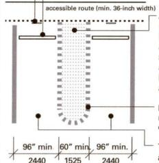
Access aisle of at least 60-inch width must be level (1:50 maximum slope in all directions), be the same length as the adjacent parking space(s) it serves and must connect to an accessible route to the building. Ramps must not extend into the access aisle.
